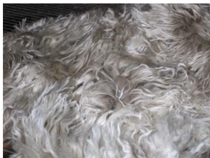
Picture 7 22um suri , 120mm length used to produce the fabric in NZ trial
